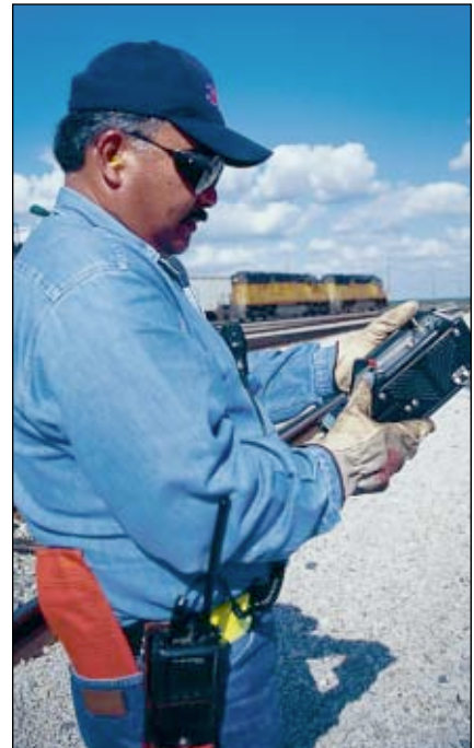
Brakeman Mike Gonzalez operates a remote-control switch to realign track and permit smooth train operations in the rail yard.
